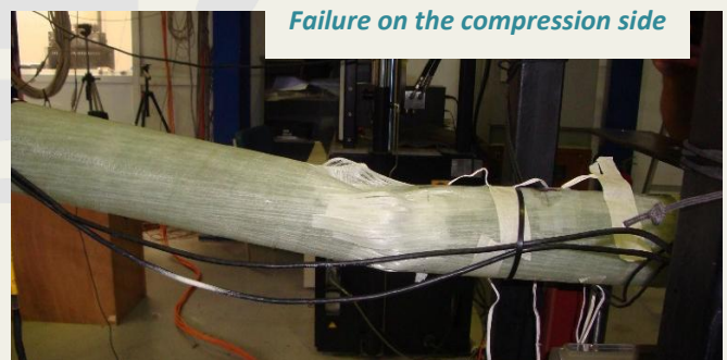
Experimental GFRP pole before load application - Failure on the compression side
