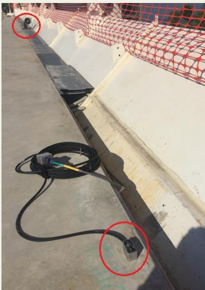
Fig. 2 - Position, numbering and cabling of sensors
