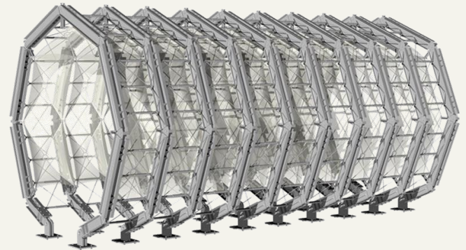
Fig. 1 The concept of a shape-controlled building by [Christoforou et al., J. of Mech. Design 137 (4), 2015] – Robotics' principles are combined with design principles of lightweight structures as bar linkages are interconnected through an arrangement of telescoping members and diagonal cables/pulleys, which transform the typical frame of the building, while membranes are used for creating an envelope.
