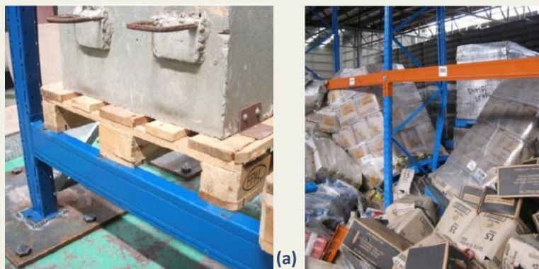
Fig. 2 (a) Content sliding along the cross-aisle direction (Castiglioni et al., 2018) and (b) rack collapse due to pallet falling off (Clifton et al., 2011).
