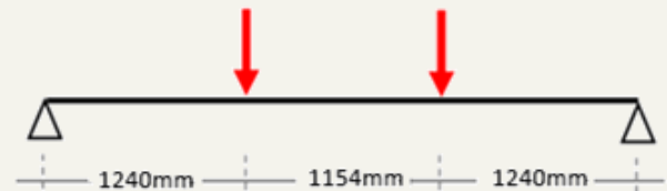
Fig. 2 Simply-supported purlin and locations of load application
