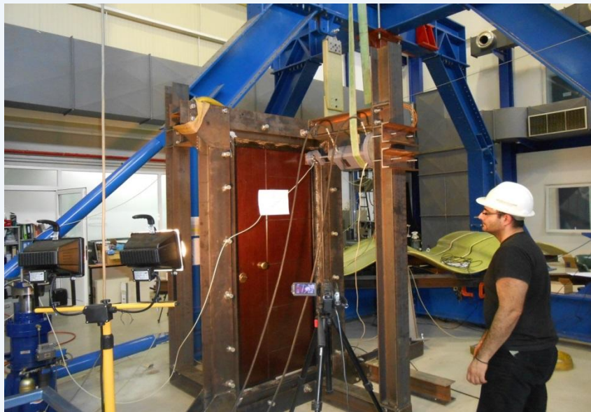
Static tests to EN 1628
