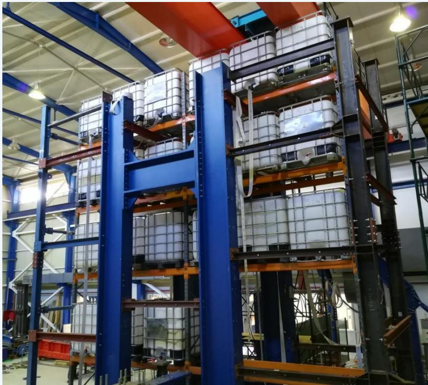
Static test under horizontal loading
