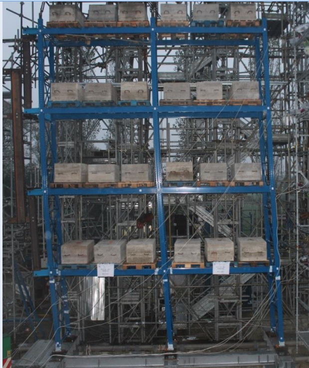
Fig.1 Typical unbraced racking system in full scale test
